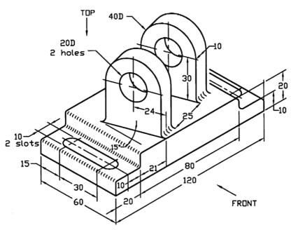
Draw the isometric view of the guide bracket as shown below. Put the top, front and RS View on a drawing sheet.
